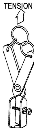
FIG. 5 Tension Test Adaptor/Clamp
